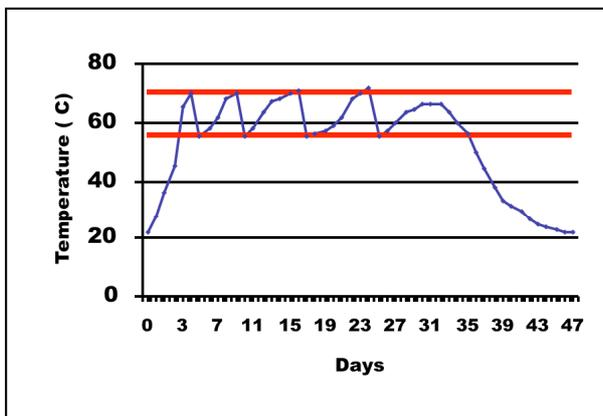
The temperature cycle of the compost heap will follow a similar trend to that displayed in the graph. The temperature will continue to rise until the pile is turned, when it temporarily drops. It then slowly begins to rise again. This will continue until all the nitrogen in the pile has been utilized. If your compost does not get hot it generally indicates that there is not enough nitrogen present.
